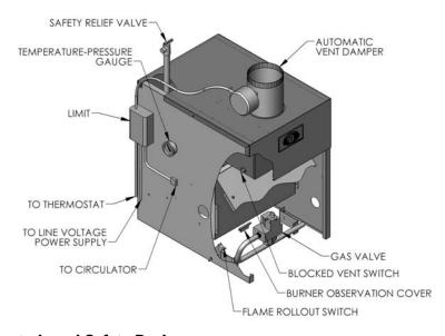
Figure 6.1: Wiring, Controls and Safety Devices
